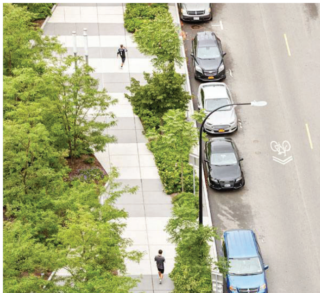
Sidewalks with continuous landscaping provide added protection from vehicles and stormwater and ecology benefits.
