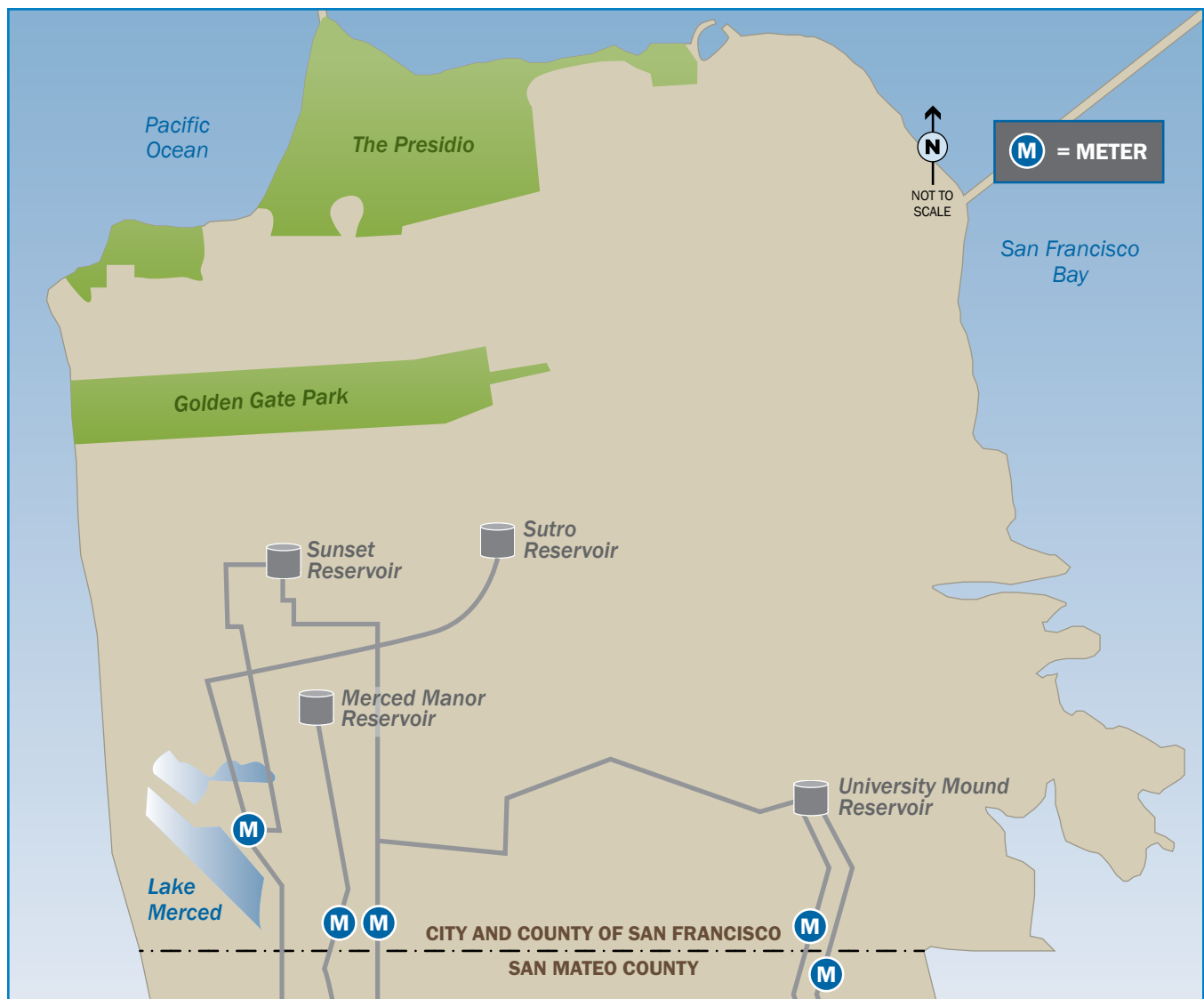
Figure 7: Distribution System Area and Metering Locations
