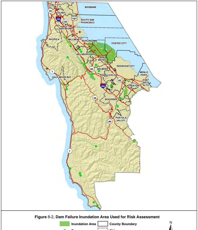
Figure 8-2. Dam Failure Inundation Area Used for Risk Assessment
