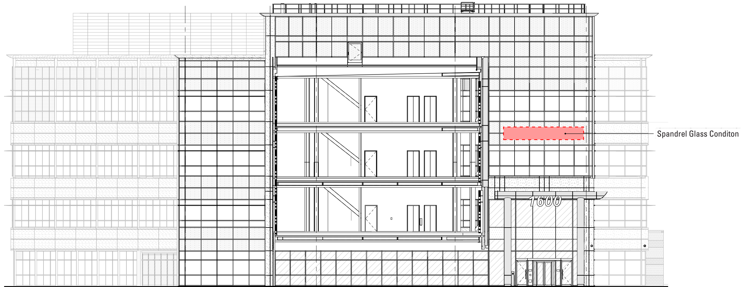
North Elevation: B3: 25' x 4', mounted to building facade
