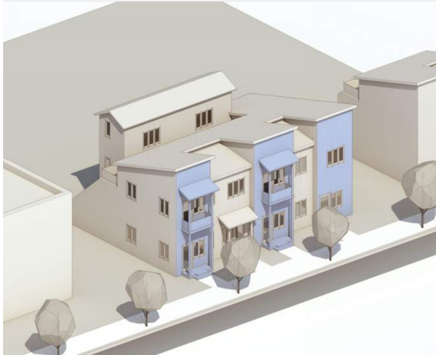
Figure 7. At least 40% of the planes of the exterior walls along public streets shall vary in depth and/or direction (see K at right).
