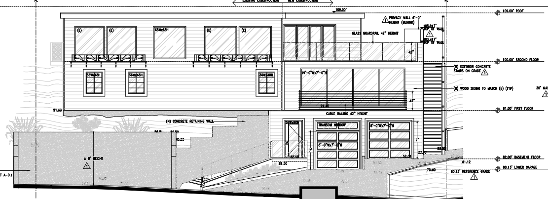
1'. (N) NORTH (FRONT) ELEVATION 1/4"=1'-0"
