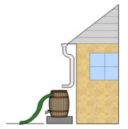
a roof downspout for non-potable, exterior uses, such as irrigation. Using rain barrels to temporarily store and reuse rainwater can conserve drinking water by providing a supplemental water source for outside landscaping. Rain barrels come in a wide variety of materials, designs, and colors. Common sizes for residential use are 55 and 90 gallons. They are typically installed on firm, level ground next to buildings.
